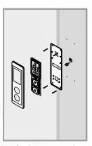
Surface mounted landing operator panels
